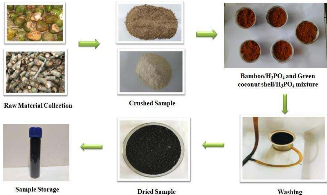
Figure 1. Flow of processing of raw materials to AC
