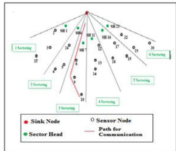
Figure 6. Static sectoring scheme for reliable data communication.
