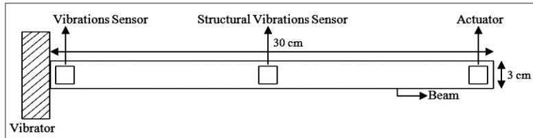
Fig. 3. Block Diagram of Cantilever beam with PZT Patches.
