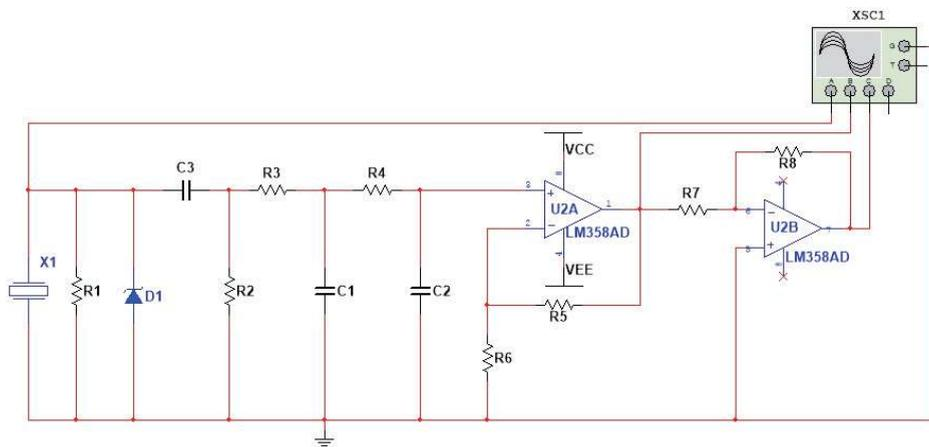
Fig. 5. Vibration Sensor Along with Inverter Circuit.
