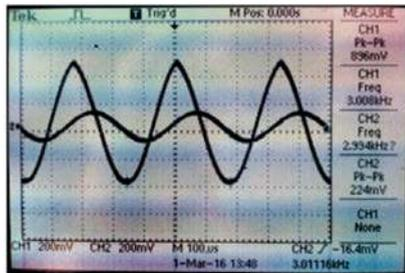
Fig. 7. Output of the System for  $D = 28$  cm.
