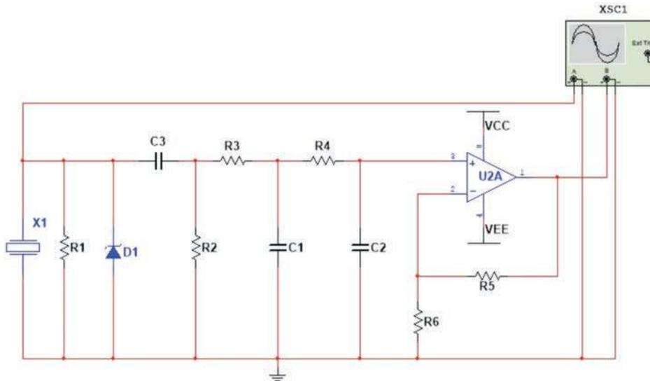
Fig. 4. Vibration Sensor Circuit.
