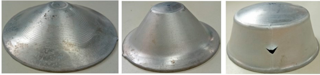
Fig. 3 Conical frustums having wall angle of 30°, 50° and 70° formed using HISF process
