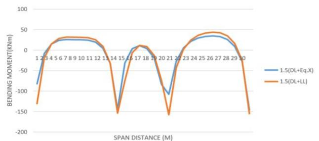
Fig. 12. For flat slab 1.5(DL+Eq.X) with 1.5(DL+LL) for R=5.
