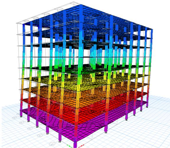
Fig. 7. Seismic load view for Flat slab building.
