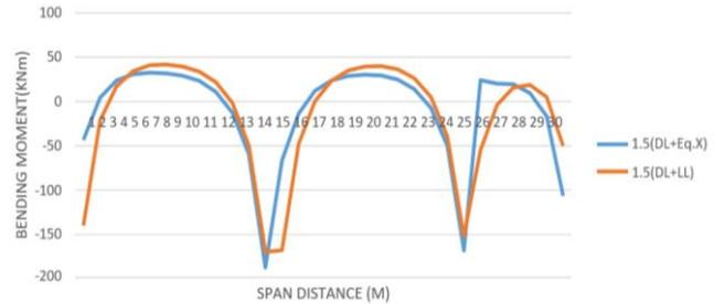
Fig. 9. For flat slab 1.5(DL+Eq.X) with 1.5(DL+LL) for R=2.
