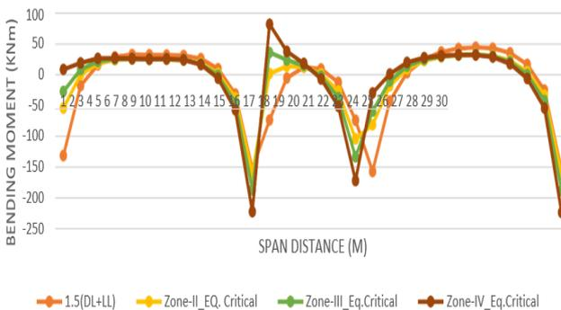
Fig. 16. For flat slab 1.5(DL+Eq.X) with 1.5(DL+LL) for R=3, Zone-II, III, IV.
