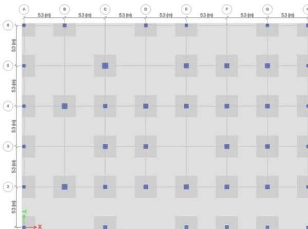
Fig. 3. Model plan drop view for Flat slab building.
