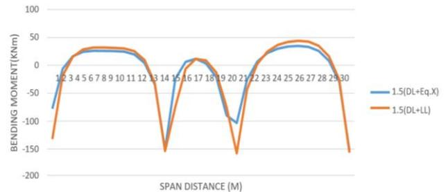
Fig. 11. For flat slab 1.5(DL+Eq.X) with 1.5(DL+LL) for R=4.
