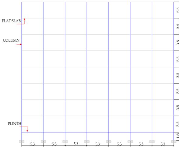
Fig. 2. Elevation of Flat slab building.
