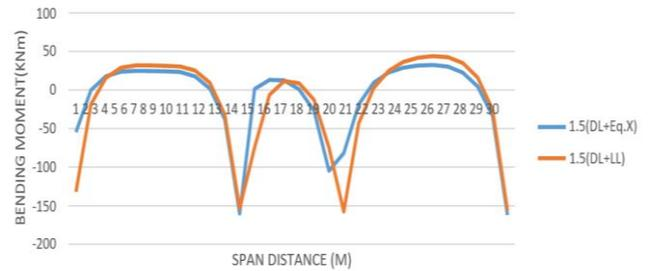
Fig. 10. For flat slab 1.5(DL+Eq.X) with 1.5(DL+LL) for R=3.
