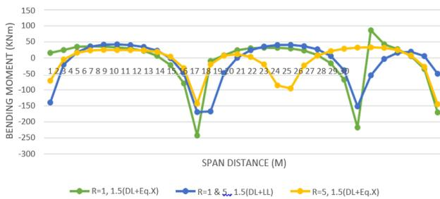
Fig. 15. For flat slab 1.5(DL+Eq.X) with 1.5(DL+LL) for R=1 Vs R=5.
