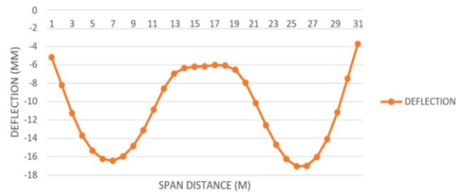
Fig. 18. For flat slab deflection Vs span dist. For R-3 & zone-II.
