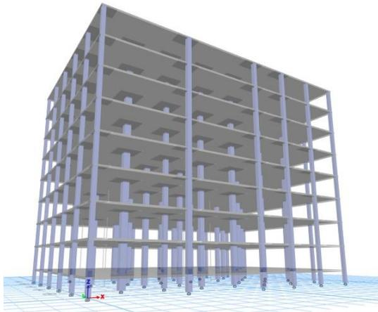
Fig. 6. Model 3D view for Flat slab building in ETABS.
