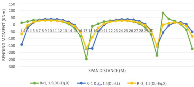
Fig. 14. For flat slab 1.5(DL+Eq.X) with 1.5(DL+LL) for R=1 Vs R=3.
