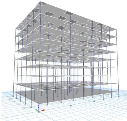
Fig. 5. Isometric view for Flat slab building in ETABS.
