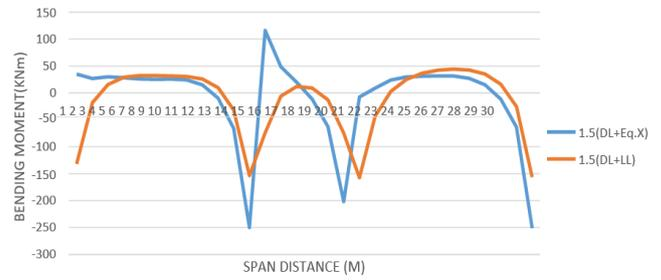
Fig. 8. For flat slab 1.5(DL+Eq.X) with 1.5(DL+LL) for R=1.
