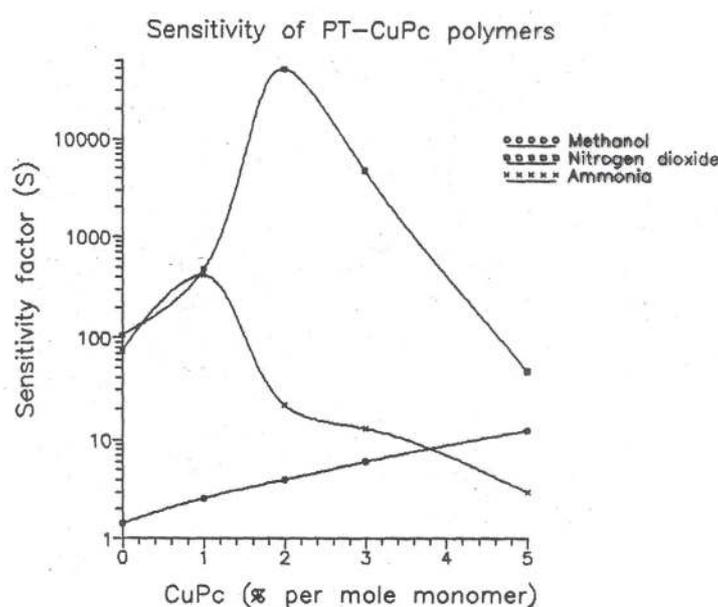
**Figure 6.** Plots of sensitivity factor versus CuPc concentration for Methanol, ammonia and nitrogen dioxide vapors measured with PT-CuPc/ PEO/ CuCl<sub>2</sub> inter-digited electrodes.
