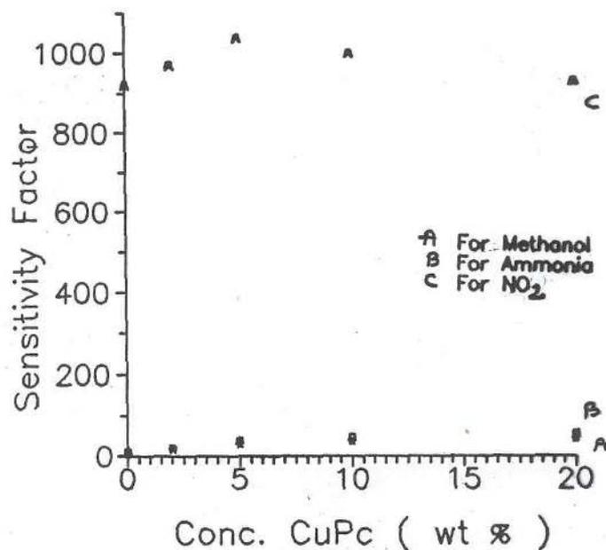
**Figure 4.** Plots of sensitivity factor versus CuPc concentration for (A) Methanol (B) Ammonia (C) Nitrogen dioxide vapours with PANI-CuPc/ PEO/ CuCl<sub>2</sub> Inter-digited electrodes
