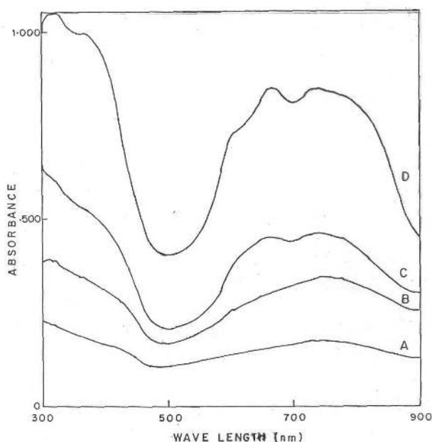
**Figure 3.** UV-VIS spectrum of PANI-CuPc polymers in dil.  $H_2SO_4$  (A) Pure PANI (B) PANI + 3% CuPc (C) PANI + 10% CuPc and (D) PANI + 20% CuPc.
