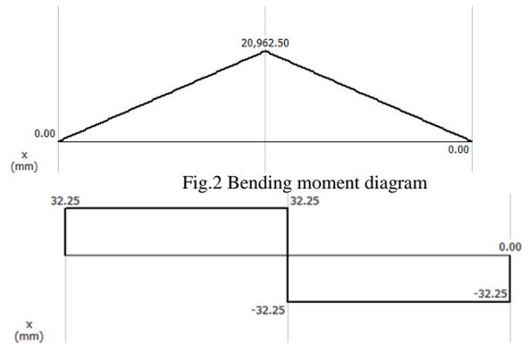
Fig.2 Bending moment diagram
