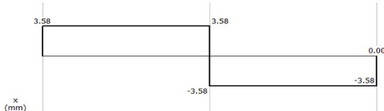
Fig.6 Shear diagram
