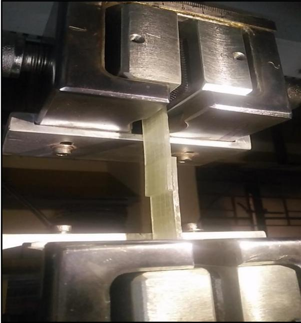
Fig. 1 Fatigue test of bonded joint.
