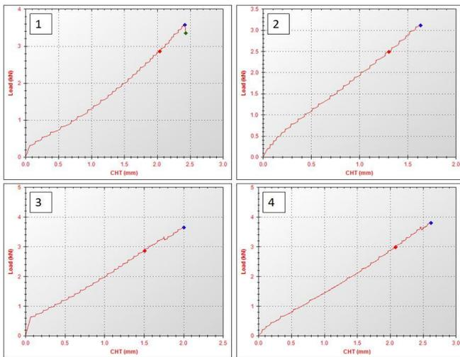
Fig 4. Load Displacement Curves for the Composite Joint.
