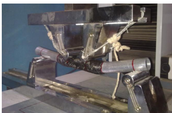
Figure 4.2 Photograph of the flexural loading
