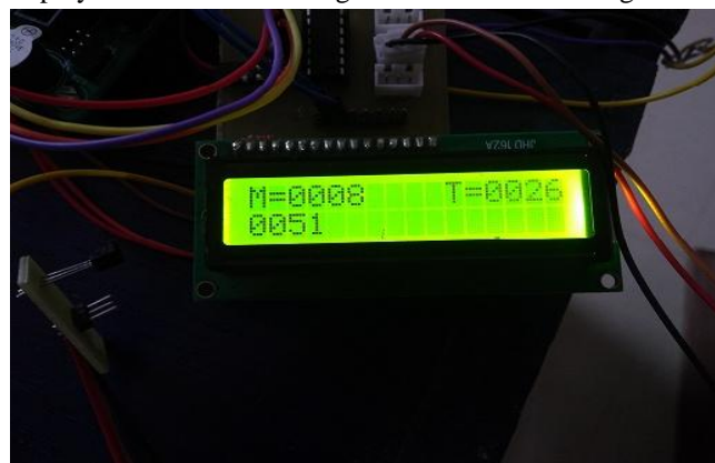
Figure 6: LCD displaying the sensor output at the transmitting end of CAN network
