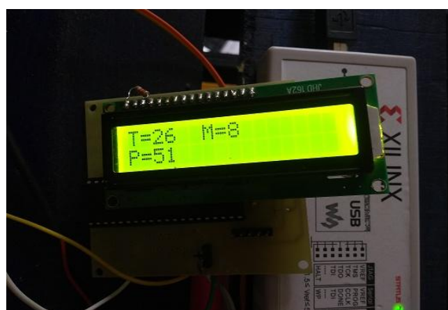
Figure 7: LCD displaying the sensed output at the receiving end of CAN network
