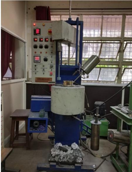
Fig. 1. Stir casting setup.
