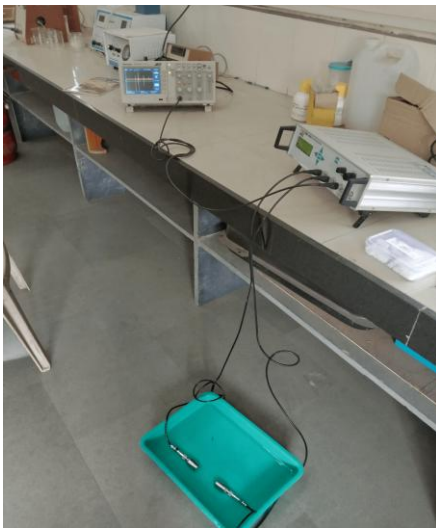
Fig. 4. Hardware setup for Non-Destructive Evaluation in through transmission mode, Courtesy: Cummins College of Engineering Pune
