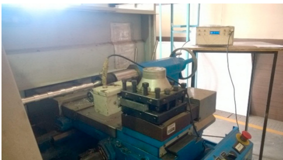
Fig. 1. Experiment setup of roller burnishing process.
