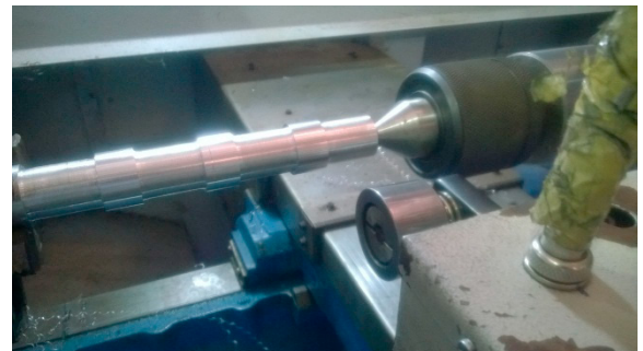
Fig. 1. Experiment setup of roller burnishing process.
