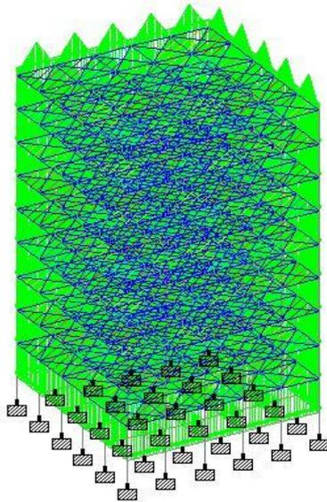
**Figure 13 Dead load diagram**
