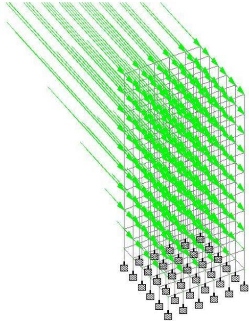
**Figure 15 Seismic load in Z direction**
