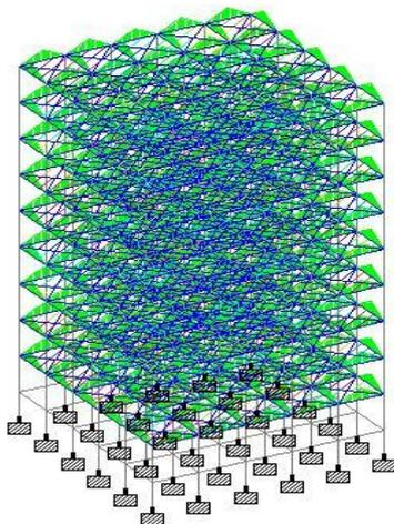
**Figure 14 Live load diagram**
