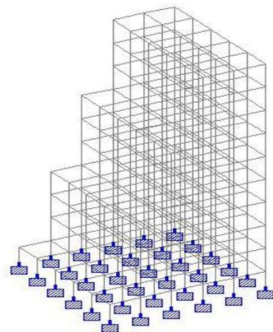
Figure 7 Isometric views of irregular stepped building figure
