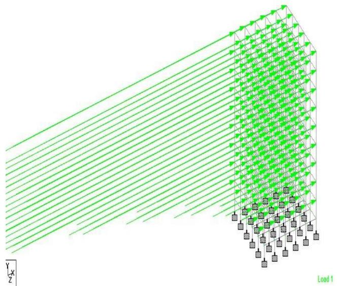
**Figure 16 Seismic load in X direction**
