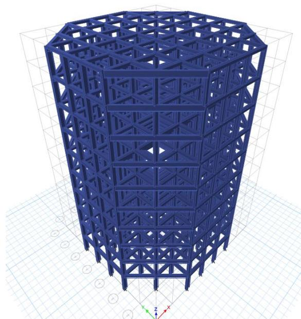
Figure 12 Isometric view of octagonal structure
