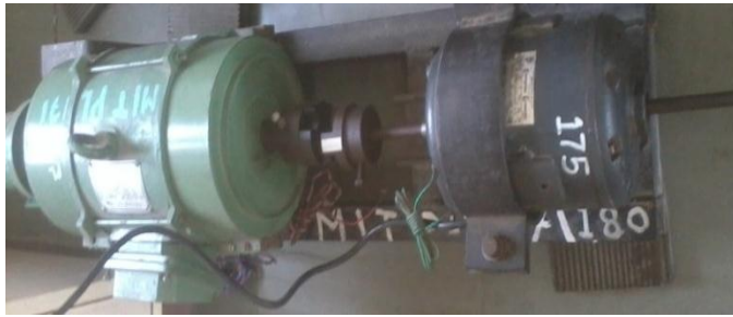
Fig. 5 - Test set up; Induction Motor # DC shunt Generator# Tacho Generator
