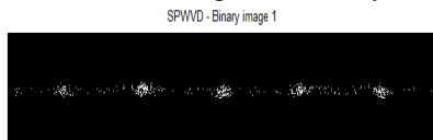
Fig. 15:- SPWVD output after Threshold – Bearing Fault
