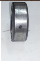
Fig. 6: - (a) Data acquisition and Hall current sensor set up (b) Bearing with fault on outer race.
