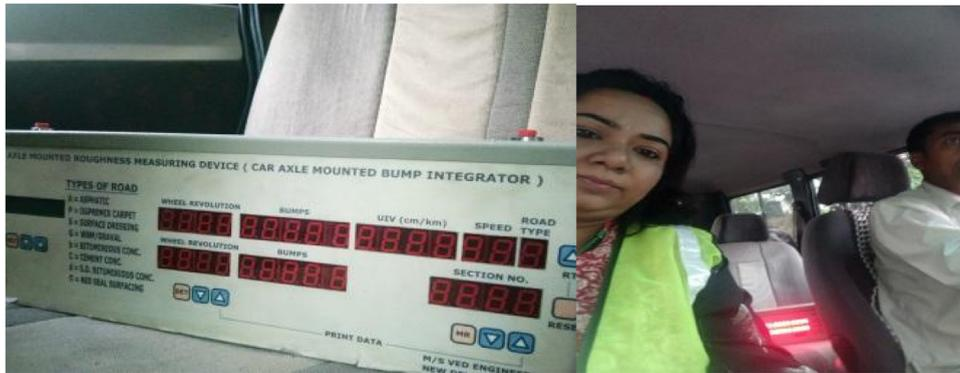
Fig. 4. Roughness test by Bump Integrator.
