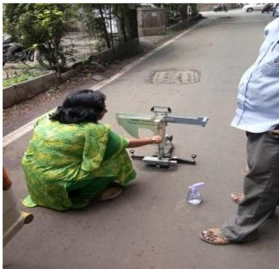
**Fig. 3.** Skid resistance using Stanley pendulum.
