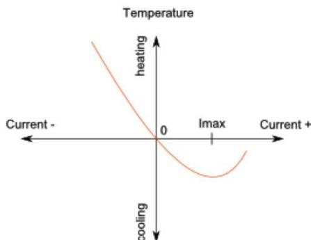
Fig 1: Effect of current on TE module
