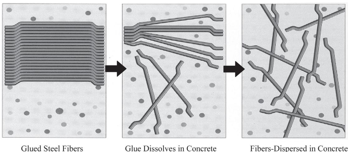
Figure 1 Dispersion of steel fibre in concrete (Bekaert-Dramix®).
