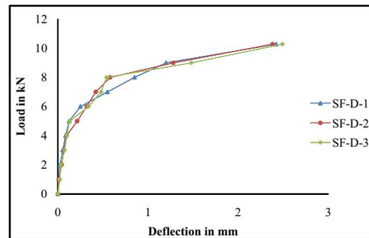
**Figure 7** SFRC beam specimens under double point loading.
