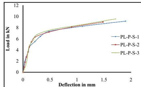
**Figure 8** Plain pre-stressed concrete beam specimens under single point loading.
