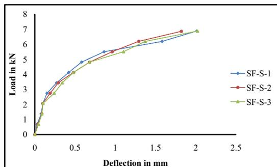
**Figure 6** SFRC beam specimens under single point loading.
