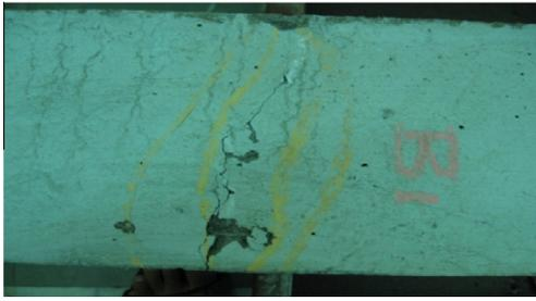
Figure 14 Crack in SFRC.
