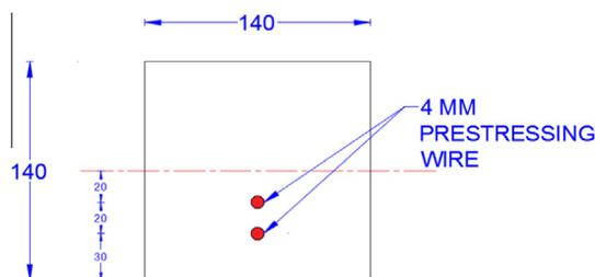
**Figure 12** Cross section of prestressed concrete beam.
