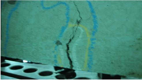
Figure 13 Crack in plain concrete.
