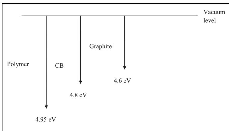
**Figure 6.** Work function diagram of PES-graphite-CB hybrid composites. PES: polyethersulfone; CB: carbon black.
