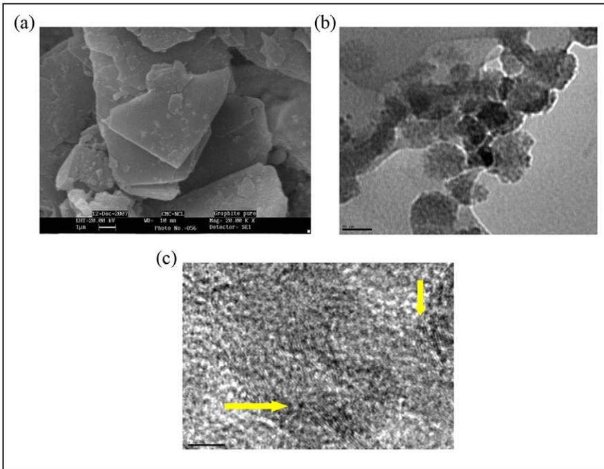
**Figure 2.** (a) SEM picture of graphite (b) and (c) TEM pictures of PES-7 wt% graphite solution-blended sample. SEM: scanning electron microscopy; TEM: transmission electron microscopy; PES: polyethersulfone.
