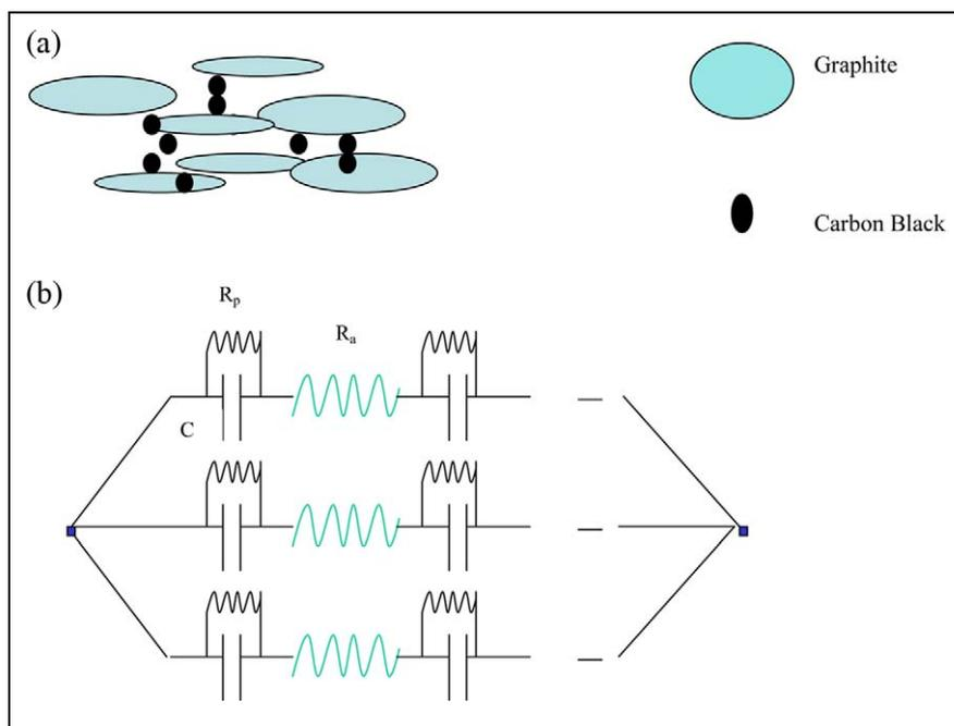
**Figure 4.** (a) Model of hybrid composites (b) equivalent circuit diagram of conducting polymer composites.
