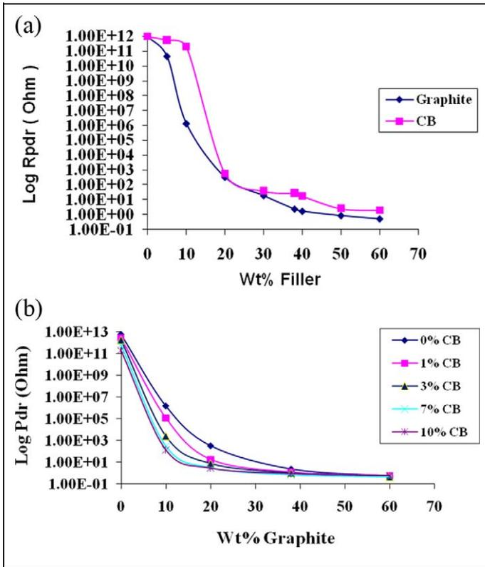
**Figure 1.** DC through thickness resistance (sample thickness: 5 mm; area: 1 cm<sup>2</sup>) variation in solution-blended (a) PES-CB and PES-graphite binary composites (b) PES-graphite-CB hybrid composites. DC: direct current; PES: polyethersulfone; CB: carbon black. CB: carbon black.
