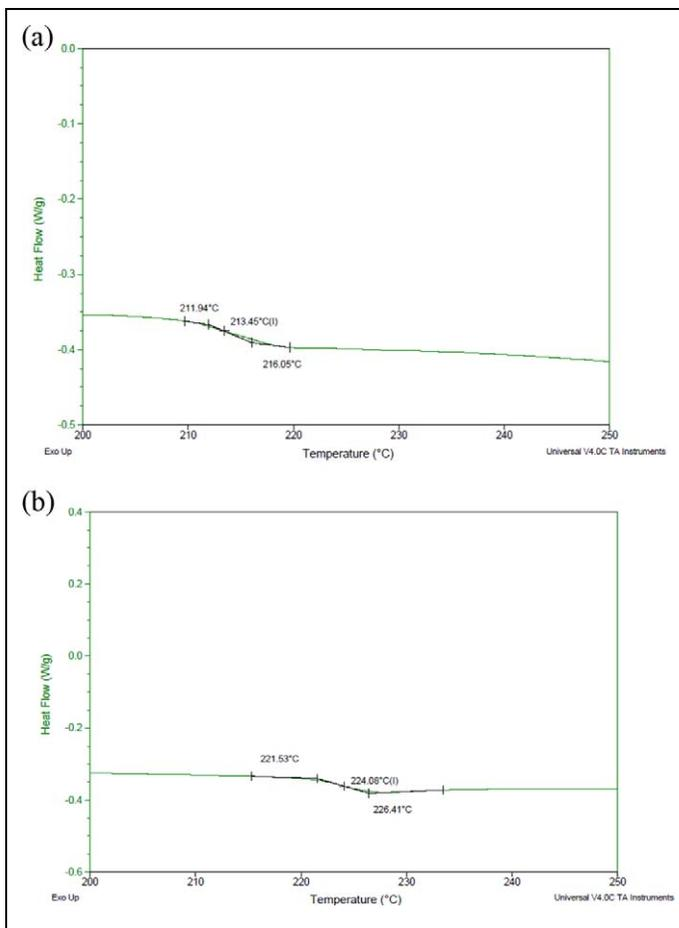
**Figure 7.** DSC curves of (a) pure PES and (b) PES-7 wt% graphite-1 wt% CB solution-blended composite. DSC: differential scanning calorimetry; PES: polyethersulfone; CB: carbon black.
