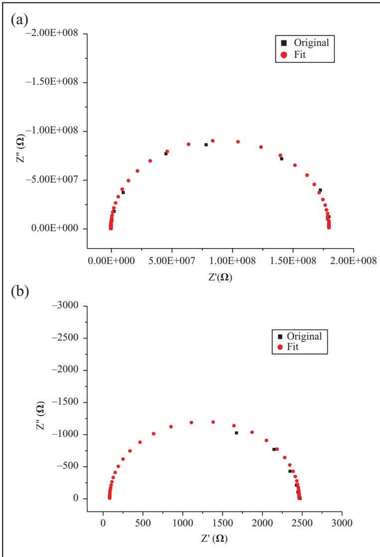
**Figure 5.** Impedance plots of (a) PES-7 wt% graphite (b) PES-7 wt% graphite-1 wt% CB solution-blended composites. PES: polyethersulfone; CB: carbon black.
