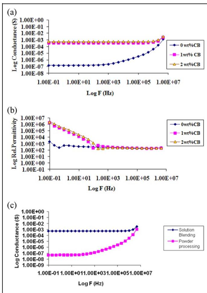
**Figure 3.** (a) AC conductance (b) effective dielectric constant variation in PES-7 wt% graphite- $x$  wt% CB ( $x = 0, 1, 2$ ) solution-blended composites, and (c) comparison of processing routes of PES-7 wt% graphite-2 wt% CB. AC: alternating current; PES: polyethersulfone; CB: carbon black.
