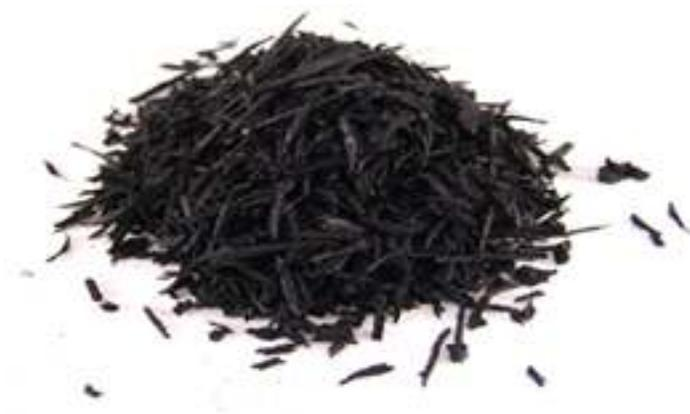
**Fig 1.** Shredded rubber tyre
