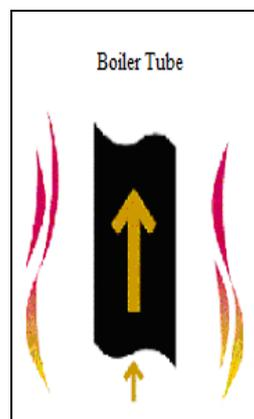
**Figure 2.** Riser fluid flow
