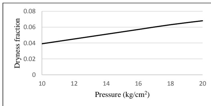
**Figure 6.** Effect of pressure on acceptable dryness fraction
