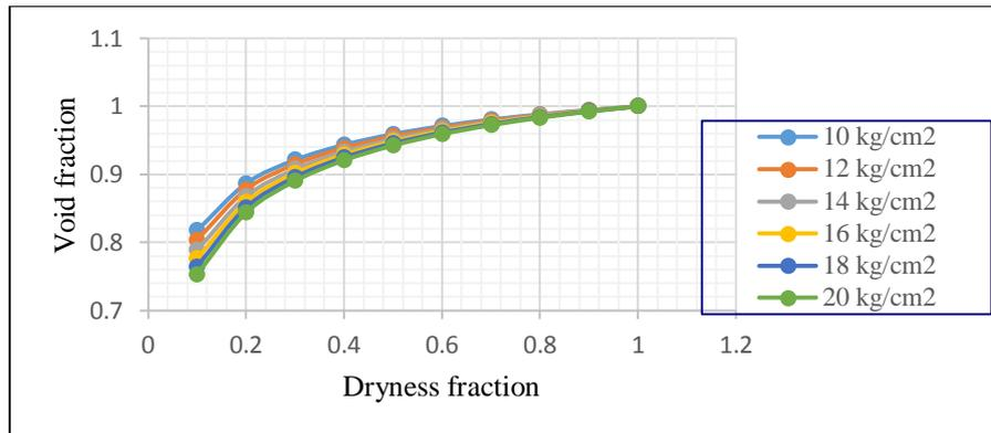
**Figure 5.** Void fraction Vs Dryness fraction
