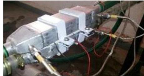
**Fig.7** Assembly of heat exchangers with modules
