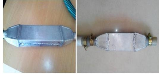
**Fig.6** Aluminium Welding of Heat Exchangers
