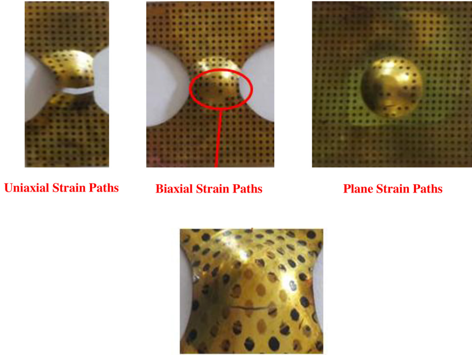
Fig. 2. Micro-formed alpha brass ultra-thin foil.
