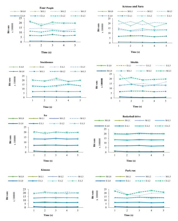
Figure 6. Comparative analysis of achieved bit rate using existing and proposed modified inter-layer dependency scheme.
