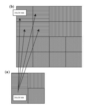
Figure 2. (a) Assignment of base bayer MB modes to enhancement layer MBs. (b) Enhancement layer MB mode derived from co-located  $16 \times 16$  MB from base layer.
