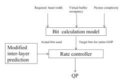
Figure 5. System structure of modified IRC algorithm with MILD.
