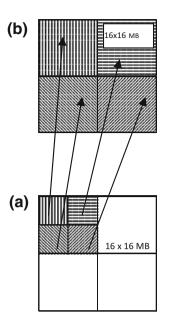
**Figure 1.** (a) Co-location of enhancement layer MB to base layer MB partition for dyadic spatial scalability. (b) Enhancement layer MB mode assigned from co-located  $8 \times 8$  block of base layer.
