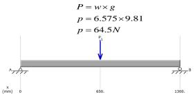
Fig.1 loading diagram
