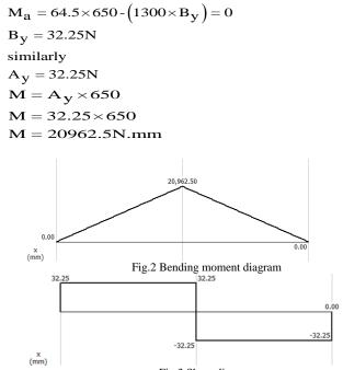
Fig.3 Shear diagram **2.3** Fatigue life prediction
