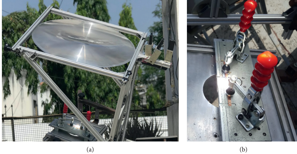
FIGURE 4: “Concentrated Solar Energy Soldering (CSES)” experimental setup.
