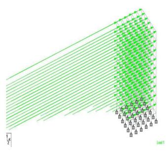
Figure 16 Seismic load in X diection
