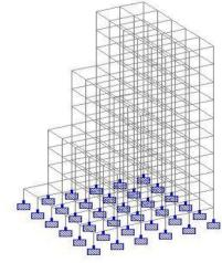
Figure 7 Isometric views of irregular stepped building figure
