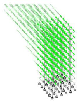
Figure 15 Seismic load in Z direction
