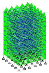
Figure 13 Dead load diagram
