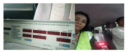
Fig. 4. Roughness test by Bump Integrator.
