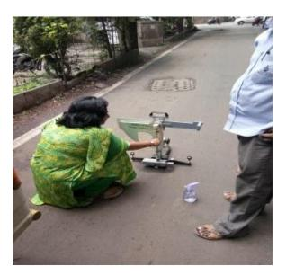
Fig. 3. Skid resistance using Stanley pendulum.
