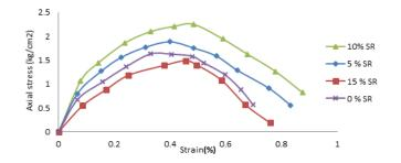
Fig 3. Stress- strain variation for untreated and shredded rubber soil
