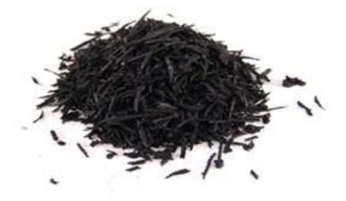
Fig 1. Shredded rubber tyre
