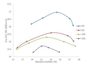
Fig 2. Dry unit weight and moisture content variation for untreated and shredded rubber soil
