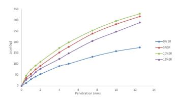
**Fig 5.** Load – penetration curve for the soil with varied % of shredded rubber
