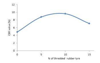
Fig 6. Variation of CBR value with different percentage of shredded rubber content in soil
