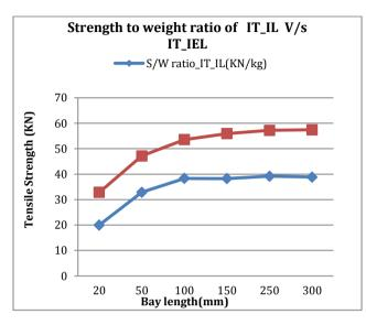
Fig.6 Strength to weight ratio for IT\_IL and IT\_IEL
