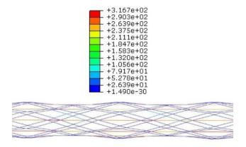
**Fig.4** Variation of Stress(MPa) developed in IsoTruss IT\_IL for 100mm bay length
