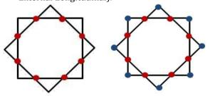
**Fig. 2** Cross Sectional view of IT\_IL(left ) and IT\_IEL(right) indicating positions of longitudinal members.
