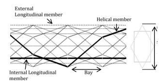
Fig.1 Parameters of 8 node configuration IsoTruss
